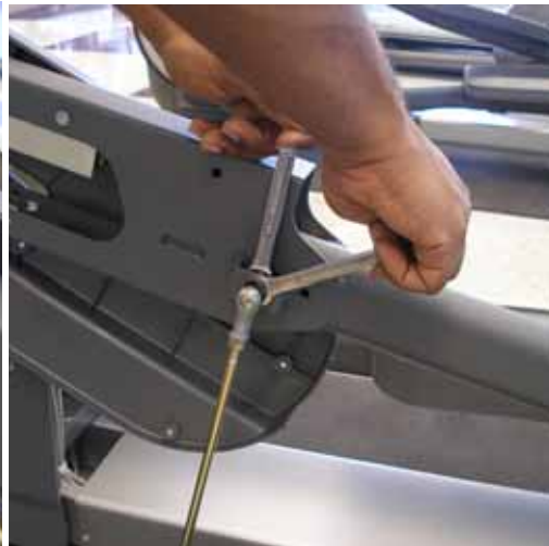
Fig. 6: removing the control link assembly
