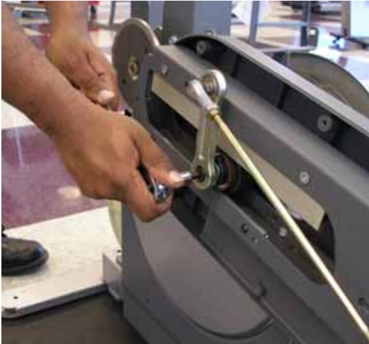
Fig. 5: removing the crank extension bolt
