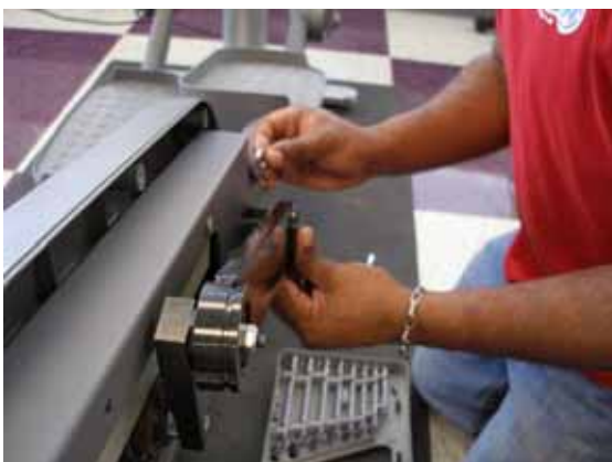
Fig. 7: use the old crank extension mounting bolt
