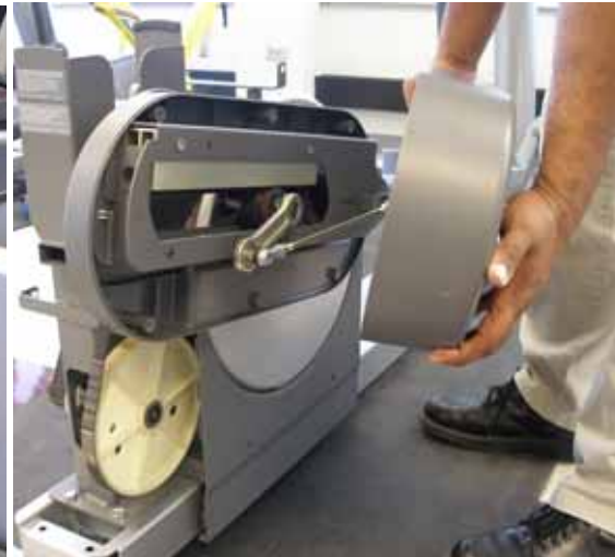
Fig. 4: removing the right outer link cover
